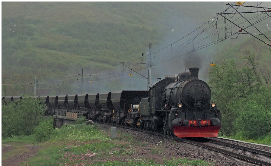
Sweden. 0-10-0 R 976 with part of an iron ore train (1,300 tonnes) at Björkliden. Immediately behind the locomotive is a match vehicle as the modern wagons have heavy duty auto-couplers. Seen on 3/7/22.
