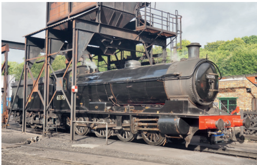
NER Q6 0-8-0 63395 stands under the coaling plant on Grosmont Shed after two return workings from Grosmont to Pickering on the North Yorkshire Moors Railway on 2/8/22.
